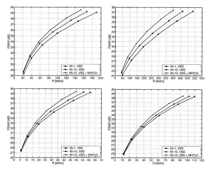
Fig. 16. Average luminance PSNR over total rate for the sequences *Foreman* (top left), *Mobile & Calendar* (top right), *Sean* (bottom left), and *Weather* (bottom right). The performance of the multihypothesis codec with VBS and long-term memory motion compensation is shown.
