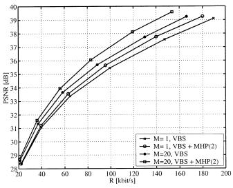
Fig. 14. Average luminance PSNR over total rate for the sequences *Foreman*. The performance of the multihypothesis codec with VBS is depicted for M=1 and M=20 reference frames.
