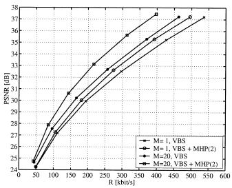
Fig. 15. Average luminance PSNR over total rate for the sequences *Mobile & Calendar*. The performance of the multihypothesis codec with VBS is depicted for M=1 and M=20 reference frames.
