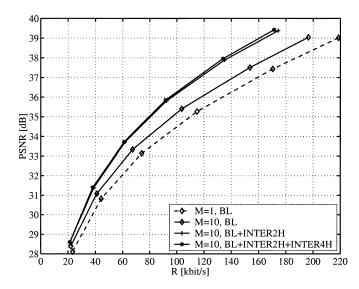
Fig. 8. Average luminance PSNR over total rate for the sequence Foreman depicting the performance of the multihypothesis coding scheme for constant block size. M=10 reference pictures are utilized for prediction.
