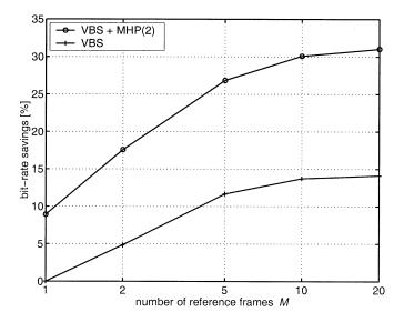
Fig. 13. Bit-rate savings at 35-dB PSNR over number of reference pictures for the sequence *Mobile & Calendar*. The performance of the multihypothesis codec with VBS is depicted for a variable number of reference frames M.
