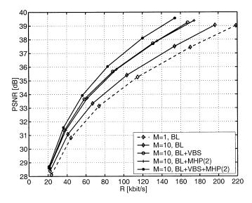
Fig. 10. Average luminance PSNR over total rate for the sequence *Foreman*. Multihypothesis and VBS prediction can be successfully combined for compression. M=10 reference pictures are utilized for prediction.
