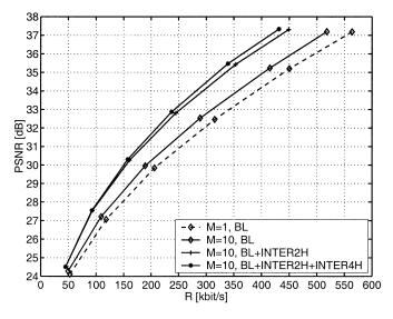
Fig. 9. Average luminance PSNR over total rate for the sequence *Mobile & Calendar* depicting the performance of the multihypothesis coding scheme for constant block size. M=10 reference pictures are utilized for prediction.
