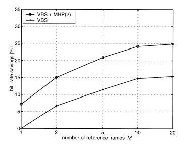
Fig. 12. Bit-rate savings at 35-dB PSNR over a number of reference pictures for the sequence *Foreman*. The performance of the multihypothesis codec with VBS is depicted for a variable number of reference frames M.
