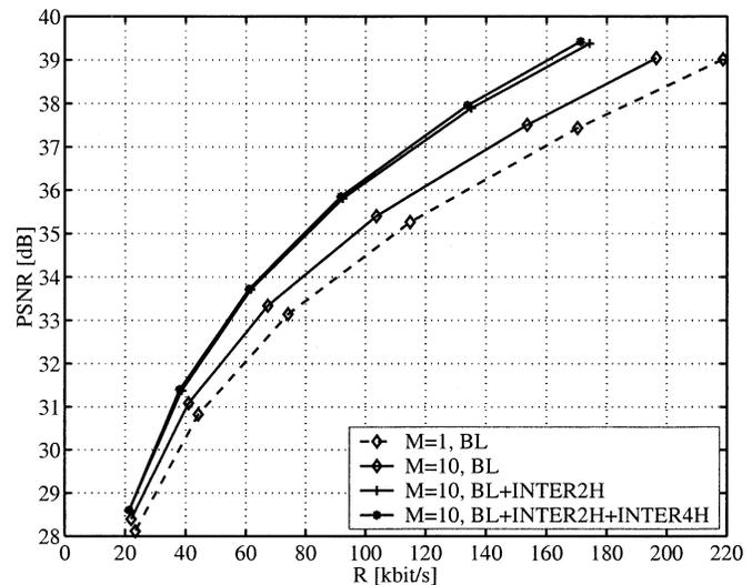
Fig. 8. Average luminance PSNR over total rate for the sequence *Foreman* depicting the performance of the multihypothesis coding scheme for constant block size.  $M = 10$  reference pictures are utilized for prediction.
