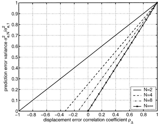
Fig. 5. Normalized prediction error variance for multihypothesis MCP over the displacement error correlation coefficient  $\rho_{\Delta}$ . Reference is the single-hypothesis predictor. The hypotheses are averaged and no residual noise is assumed. The variance of the displacement error is set very small to  $\sigma_{\Delta}^2 = 1/3072$ .
