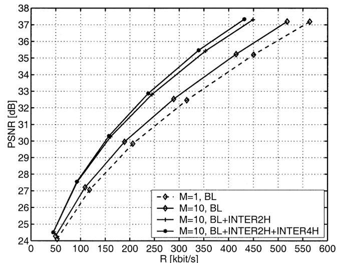
Fig. 9. Average luminance PSNR over total rate for the sequence *Mobile & Calendar* depicting the performance of the multihypothesis coding scheme for constant block size.  $M = 10$  reference pictures are utilized for prediction.
