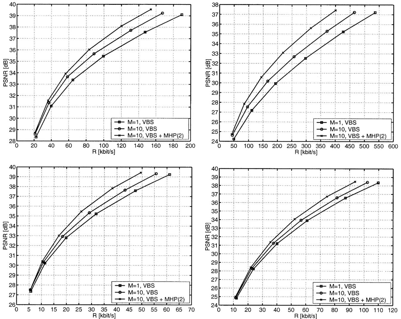
Fig. 16. Average luminance PSNR over total rate for the sequences *Foreman* (top left), *Mobile & Calendar* (top right), *Sean* (bottom left), and *Weather* (bottom right). The performance of the multihypothesis codec with VBS and long-term memory motion compensation is shown.
