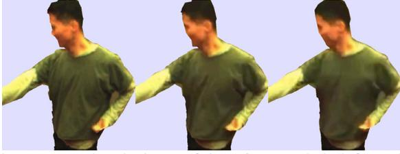
Fig. 11: Rendered views of 3DVO, uncoded (left), 1.34 Mbit/s (middle), 0.61 Mbit/s (right).
