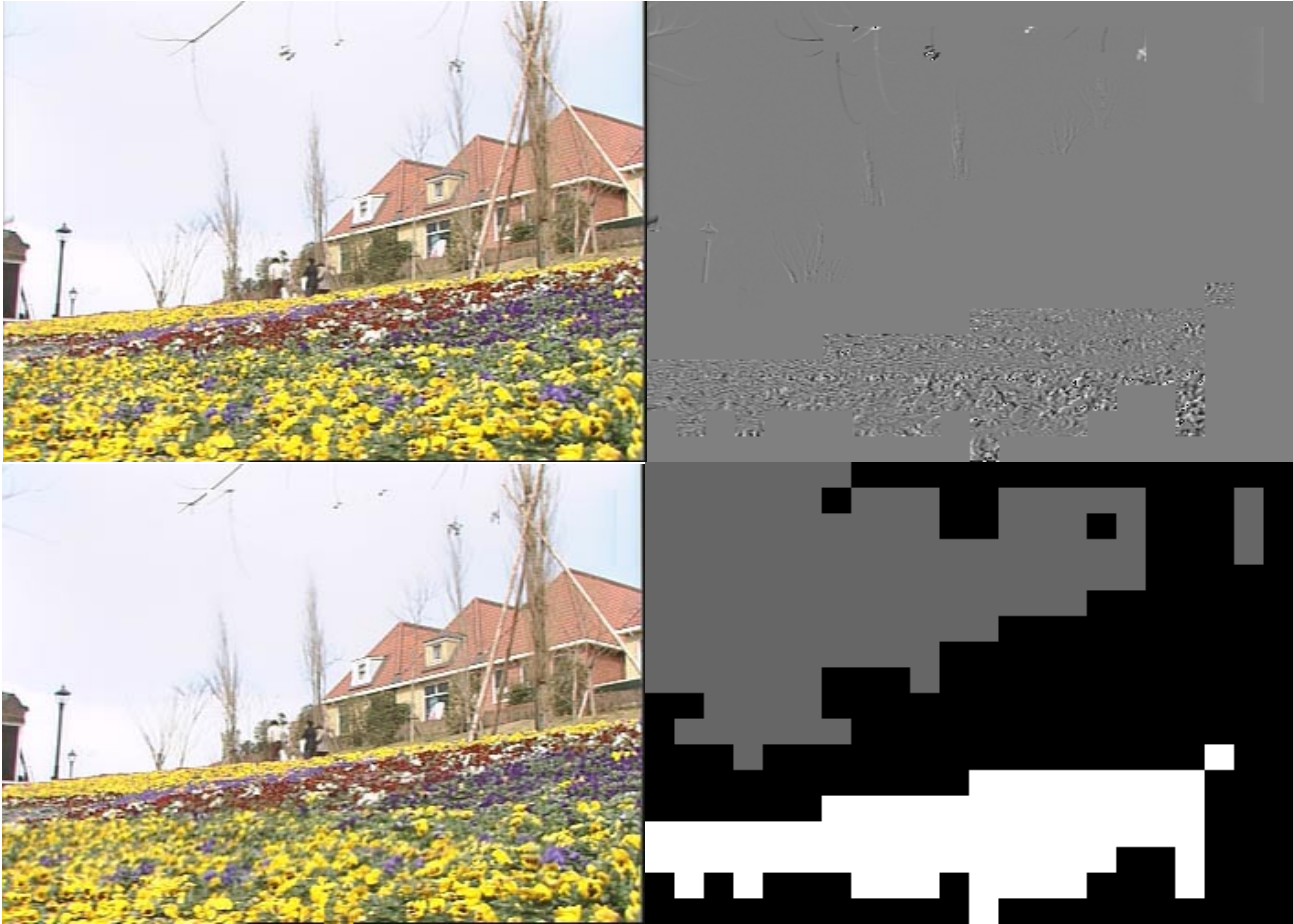
Figure 6 – Coding result for Flowergarden. Top left : Original frame (#6). Bottom left: Frame with synthesized texture regions. Top right: Difference signal (gain factor 3). Bottom right: Conservative motion compensated segmentation mask (color black corresponds to detail-relevant texture region).
