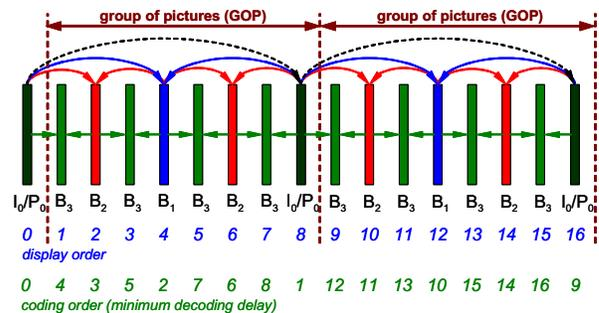
Fig. 1. Hierarchical coding structure with 4 temporal levels.
