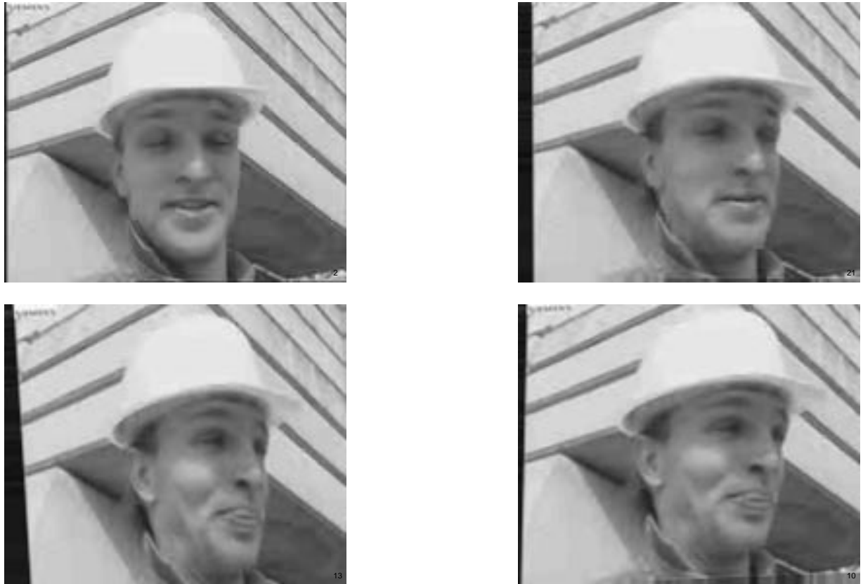
Fig. 3. Four additional reference frames. The upper left frame is a decoded frame that was transmitted 2 frame intervals before the previous decoded frame. The upper right frame is a warped version of the decoded frame that was transmitted 1 frame interval before the previous frame. The lower two frames are warped versions of the previous decoded frame.
